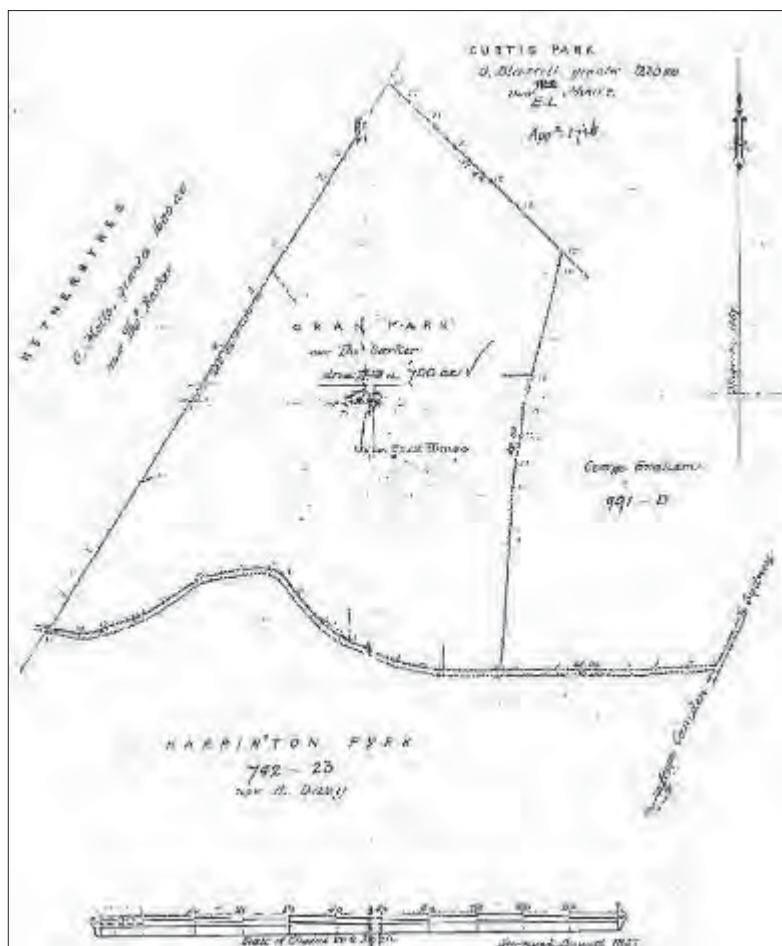
Figure 19: Titled 'Plan of Oran Park part of Wm Campbell's 2000 acres grant now the property of Thomas Barker Esq' the above diagram shows Oran Park and its neighbours as surveyed by Edward Knapp in 1867. Lands Department
