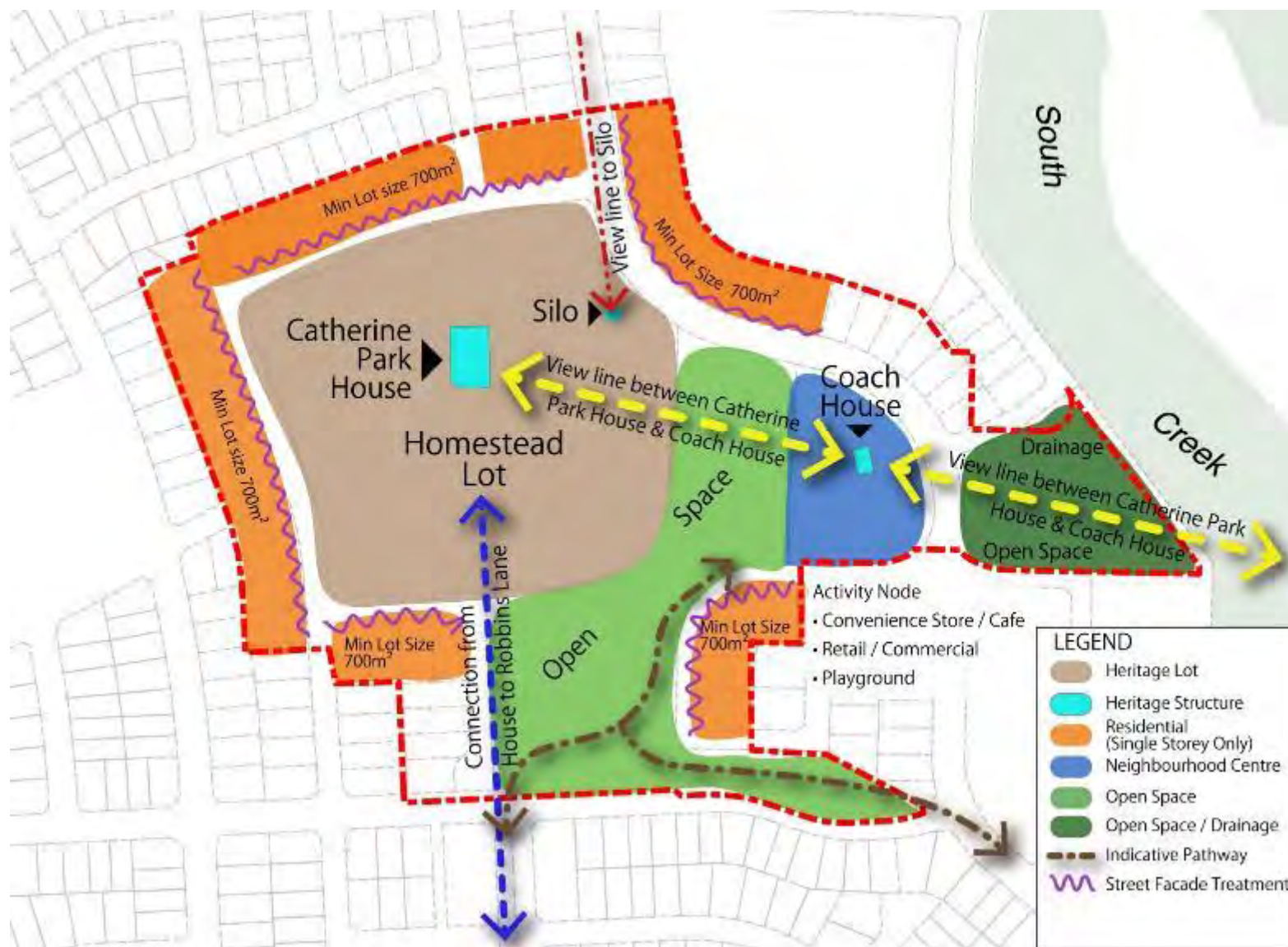
Figure 157: Oran Park outer Heritage Principles plan showing the important view lines and proposed and approved controls surrounding the Homestead Lot in the current residential subdivision of the property. This figure was prepared to inform the Heritage Exemption Guidelines and does not preclude other forms of development.
